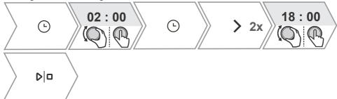
First set the cooking time. Rotate the KNOB to set the desired cooking time. Confirm the selection by pressing the KNOB. The selected oven operating time will appear on the display unit.
