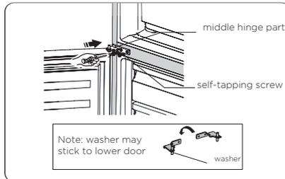
14. Transfer the upper door to the appropriate position. Secure the door`s level, make the middle hinge axis into the lower hole of the upper door.
