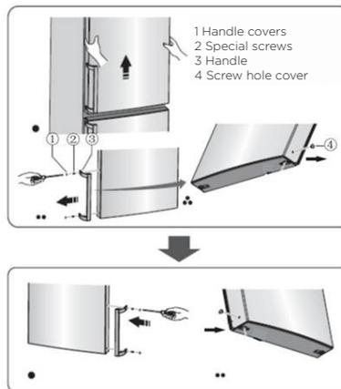
**Warning!** When changing the side at which the door opens, the appliance must not be connected to the mains. Remove plug from the mains beforehand.
