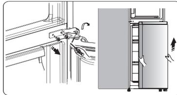
6. Place the lower door on a smooth surface with its panel upwards. Loose screw (3) and take down part (1) and part (2), then Install door stopper-left (4) (provided in the plastic bag) and left part (2) and screw (3) to the left side and tighten them securely. Keep part (1) with the appliance for future reference.
