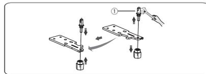
10. Change screw hole covers on lower cover plate from left to right (as shown in figure below).
