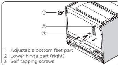
9. Remove part (1) from the lower hinge part(right), loose out the lower hinge pin, change it to the reverse hole site, and then tighten into position, then install part (1) on the lower hinge pin.
