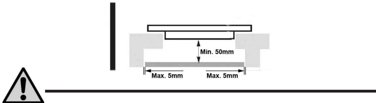
There are ventilation holes around outside of the hob. YOU MUST ensure these holes are not blocked by the worktop when you put the hob into position.
