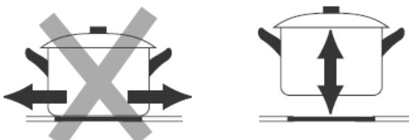
The cooking zones are, up to a limit, automatically adapted to the diameter of the pan. However the bottom of this pan must have a minimum of diameter according to the corresponding cooking zone. To obtain the best efficiency of your hob, please place the pan in the centre of the cooking zone.
