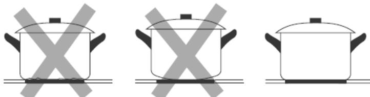
Make sure that the base of your pan is smooth, sits flat against the glass, and is the same size as the cooking zone. Use pans whose diameter is as large as the graphic of the zone selected. Using a pot a slightly wider energy will be used at its maximum efficiency. If you use smaller pot efficiency could be less than expected. Always centre your pan on the cooking zone.
